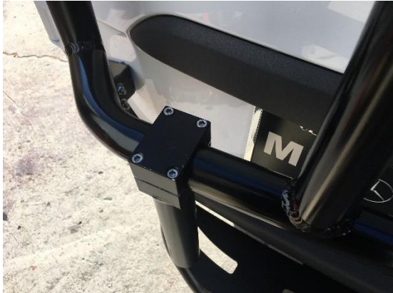
Figure 14: Bolt-On Supports Loosely Bolted to Lower Crossmember
