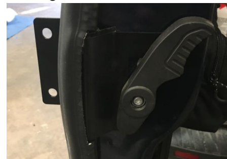
Figure 13: Installed Weather Stripping After Modification
