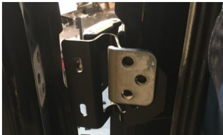
Figure 3: Bracket Installed Over Factory Hinge
