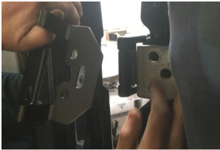
Figure 2: Upper Hinge Rotated Away from Door
