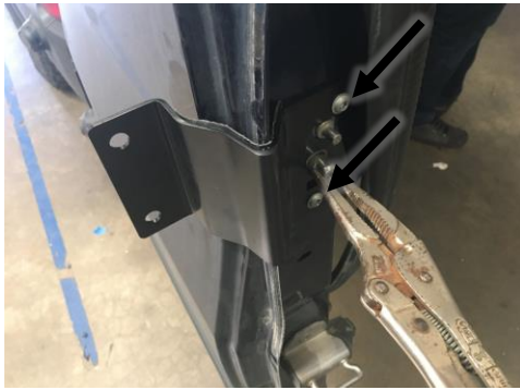
Figure 9: Inner Driver Door Bracket Installed
