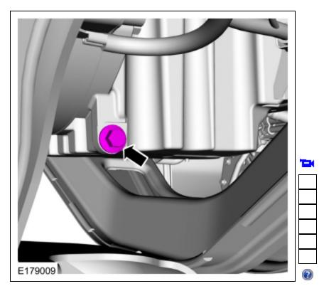
3. Remove and discard the engine oil filter. Use the General Equipment: Oil Drain Equipment
